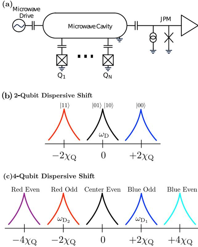
FIG. 1. (Color online) (a) Schematic of the experimental design showing the cavity,  $N$  coupled qubits, and the photon counter (a JPM in this case). (b) and (c) Illustration of the dispersive shifts on the cavity for two- and four-qubit computational basis states.
